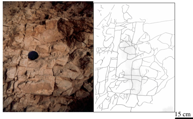
(b) Outcrop: A producing formation (limestone) in Field 5 upper formation (photo and fracture trace map).
