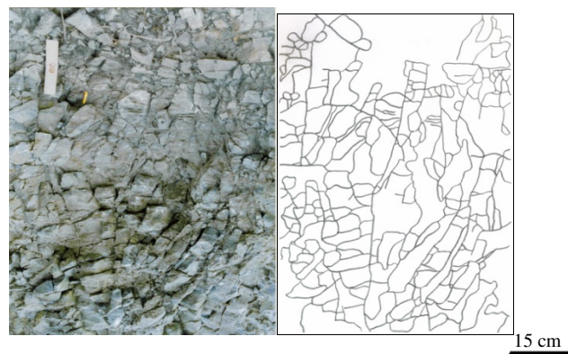
(c) Outcrop: A producing formation (marble) in Field 1 (photo and fracture trace map).
